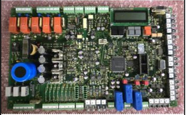
A photograph of a green printed circuit board (PCB) labeled 'PCB power control V1.2'. The board is densely populated with electronic components, including integrated circuits, resistors, capacitors, and a large blue cylindrical component. It features a central processing unit (CPU) and various connectors.  |
