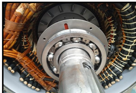
Fig. 4. DE Bearing renewal.
