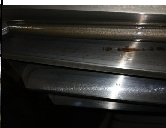
Obs: adhesion, abrasion and micropitting
