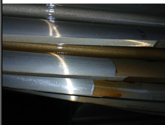
Obs: adhesion, abrasion and micropitting
