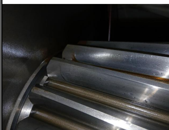
Obs: adhesion, abrasion and micropitting
