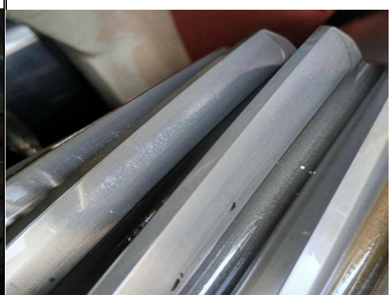
Obs: adhesion, abrasion and micropitting
